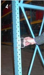
Place an H591 Connector into the holes selected for the first Beam level. In photographs 4 and 5, the Connector is shown being inserted through the holes from the backside of the Column and held in place as the Beam is positioned.
