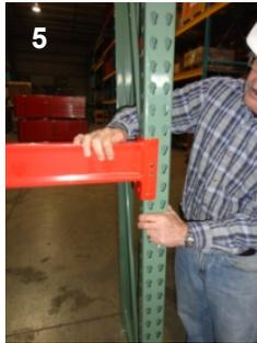
Seat the Beam, as shown in photographs 4 and 5, by engaging the studs in the beam end plate into the keyholes of the column. The beam is correctly seated when the H001 Spring Clip slides into the top of the end plate and can then be locked in place by inserting the stud into the hole in the end plate and column as show in photograph 6.
