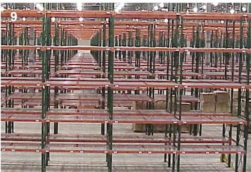
Additional rack bays and beam levels may be added as shown in photograph 9. The rack unit is now completed and Row Spacers, if desired, may be installed. Row Spacers are used to space rack rows placed back to back. They also act in distributing forces should the rack be struck. Row Spacers should always be installed in line with, or near a Horizontal Truss member, as shown in photograph 10.
